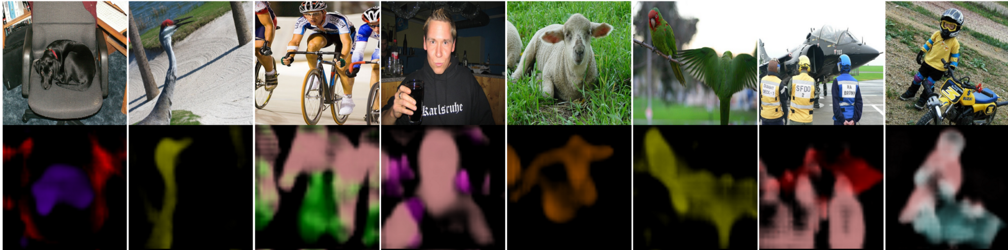
Figure 33: Semantic Segmentation priors produced by a ResNet38d model trained with OC-CSE. CAMs were generated using Grad-CAM and Test-Time Augmentation (TTA). Source: keras-explainable/wsol .
