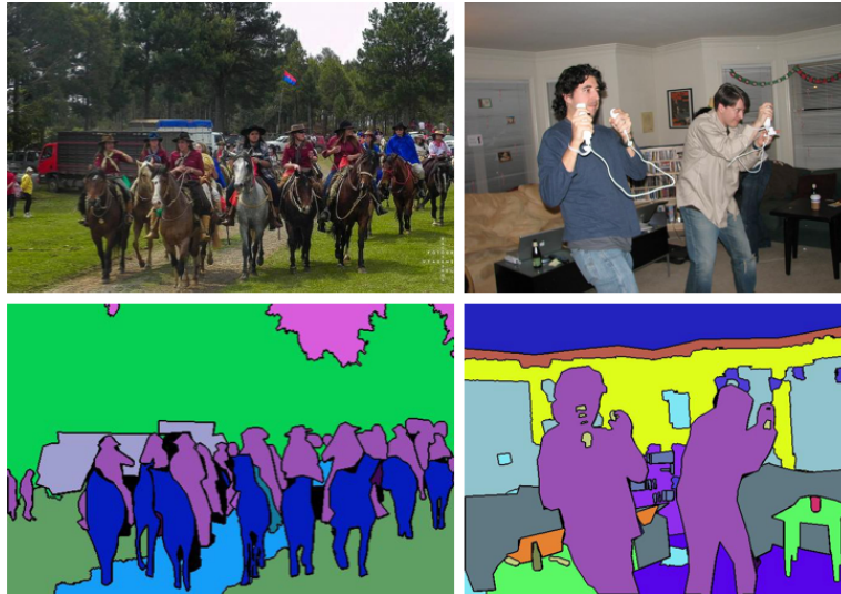
Figure 11: Example of samples and ground-truth panoptic segmentation annotation from the MS COCO 2017 dataset. Source: https://cocodataset.org/#panoptic-2020 .
