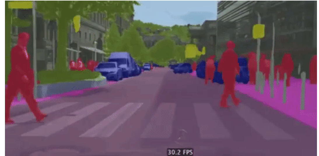
Figure 12: Example of semantic segmentation produced by ICNet for a video sample in the Cityscapes dataset. Source: https://gitplanet.com/project/fast-semantic-segmentation .
