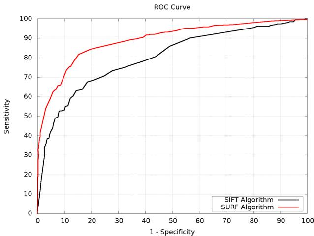
Figure 4. ROC curves using SIFT and SURF algorithms to select local features.
