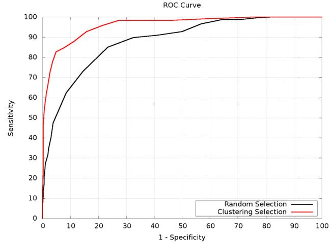
Figure 5. ROC curves using clustering and randomized selection to select the visual dictionary.
