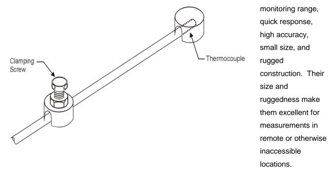
Copper-constantan (type "T") thermocouples are used because of a wide temperature
