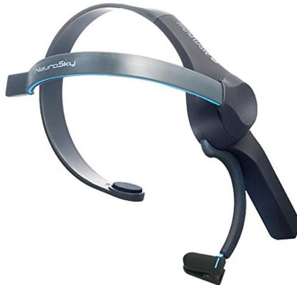
Figura 3: Headset de EEG NeuroSky Mindwave Mobile
