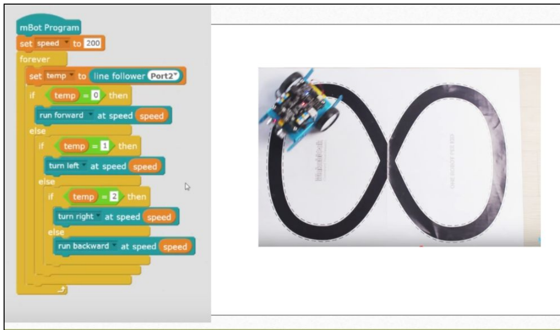
Figure 17. Second line following algorithm. Figure retrieved from “Line - following robot - mBot controlled using mBlock software” YouTube video 20 .
