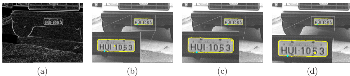
Figure 2: (a) The magnitude of the Sobel's gradient of an image for license plate detection. (b)–(d) The plate is automatically detected for different seed locations (yellow dots) using (a) as gradient-like image. The leaking pixel is always at a same place (cyan dots).
