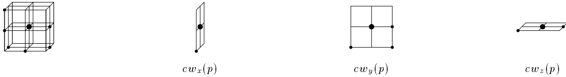
Figure 2: Example of a point p (grid central point) considered as simple by characterization 1 and non-simple by characterization 2. Note that checking windows cw_y(p) and cw_z(p) are disconnected when the central point is removed.
