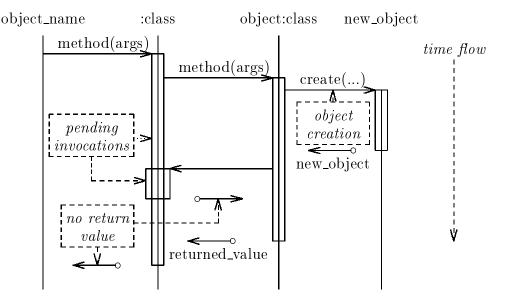
The meta-diagram above shows the subset of the UML [29] sequence diagrams notation (formerly known as interaction diagrams) we are going to use in this paper. The first lines of the diagram define one column for each object. The object may be given a name, and the class it is an instance of may be specified. A superclass name may be specified, even if the object is an instance of a subclass thereof.
