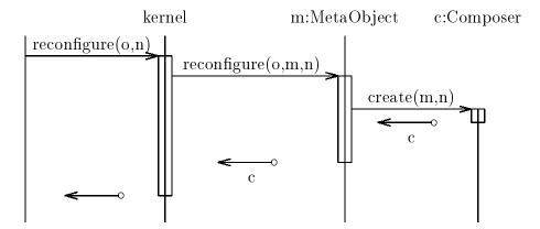
This figure shows an arbitrary object issuing a request to change the primary meta-object of object o. The requester intends to have meta-object n as the primary meta-object of o. However, meta-object m is its primary meta-object, so m is asked to decide what the new meta-configuration is going to be. It decides to create a composer c, that will delegate to both m and n, and returns this new composer, which is, from then on, the primary meta-object of object o.
