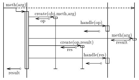
The method invocation is intercepted by the reflexive kernel. It is reified as an operation object and passed to the callee's meta-object. Eventually, the operation is delivered to the callee's application object. Then, the result of the operation is reified and presented to the meta-level similarly.
