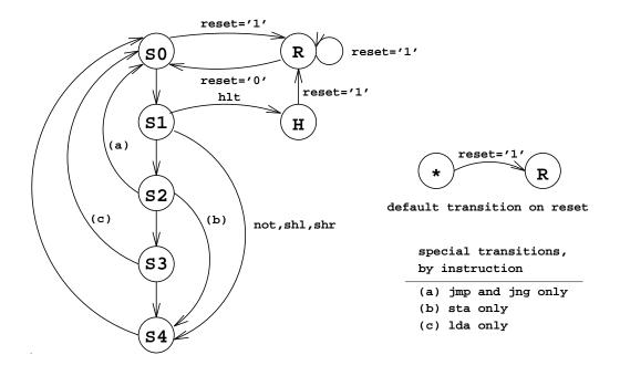
Figure 4: The State Machine Transition Diagram of CPU
