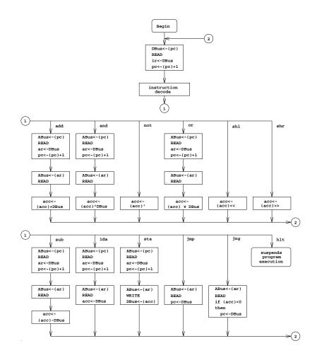
Figure 3: Micro-operations Execution Flowchart.
