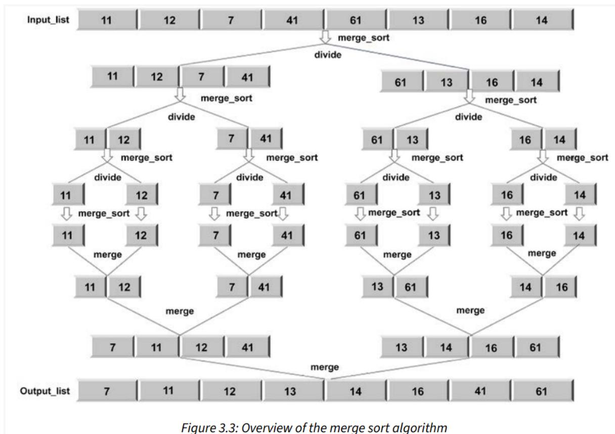
Figure 3.3: Overview of the merge sort algorithm
