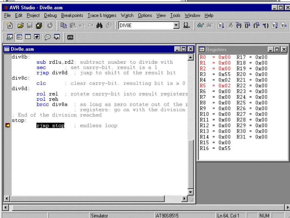
After executing the loop 16 times we have reached the breakpoint set at the end of the division routine. The result register in R5:R4 holds 0x0202, the result of the division. The registers R2:R1:R0 are empty, so we do not have a remainder left. If a remainder would have been resulted we can use it to decide whether an incrementation of the result should take place, rounding of the result up. This step is not coded here.
