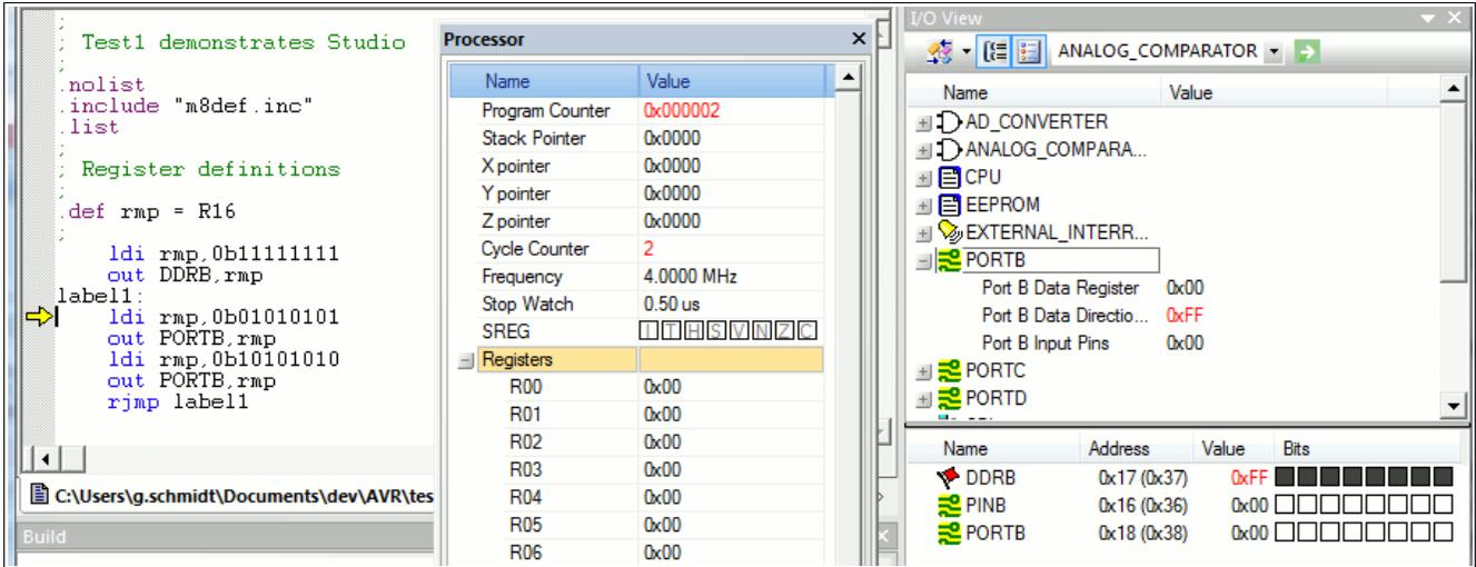
The instruction “Out DDRB,rmp” writes 0xFF to a port named DDRB. Now the action is on the I/O view window. If you push on PORTB and the small “+” left of it, this window displays the value 0xFF in the port DDRB in two different forms: as 0xFF in the upper window portion and as 8 black squares in the lower window section.
