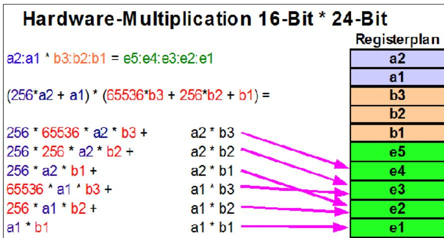
The multiplication of a 16 bit binary "a" with a 24 bit binary "b" leads to results with up to 40 bit length. The multiplication scheme requires six 8-by-8-bit multiplications and adding the results to the appropriate position in the result registers.
