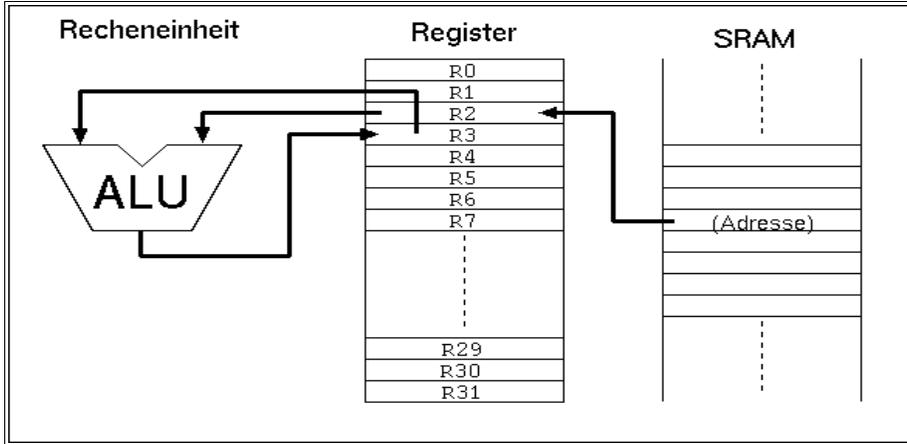
So it is clear that operations with values stored in the SRAM are slower to perform than those using registers alone. On the other hand: even the smallest AVR types have 128 bytes of SRAM available, much more than the 32 registers can hold.
