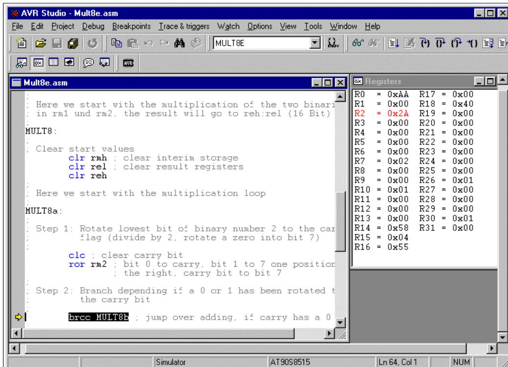
Because the carry bit had a one, the content of the registers R1:R0 is added to the (empty) register pair R4:R3, resulting in 0x00AA there.
