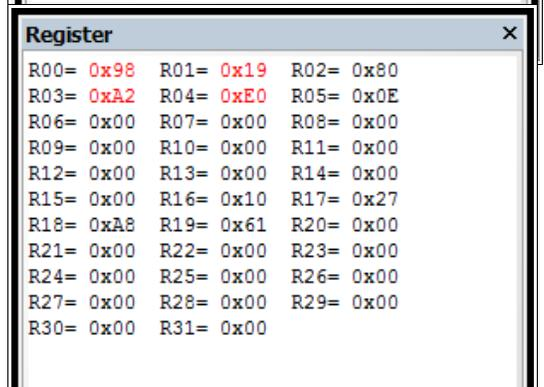
Multiplying the LSB of m1 with the MSB of m2 and adding the result in R1:R0 to the result register's two middle bytes, no carry occurred. The result is hex 0EE6B280, which is 250000000 and obviously correct ...
