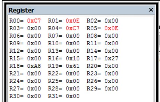
Multiplying the two LSBs (hex 10 and A8) and copying the result in R1:R0 to the two lower result registers R3:R2 ...
