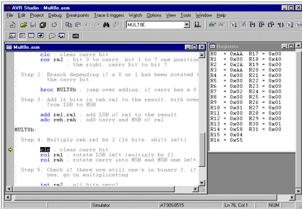
Now the register pair R1:R0 is rotated one position left to multiply this binary by 2. From 0x00AA, multiplication by 2 yields 0x0154.
