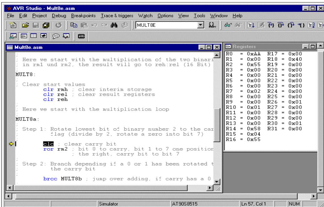
R2 is rotated to the right, to roll the least significant bit into the carry bit. 0x55 (0101.0101) yielded 0x2A (0010.1010).
