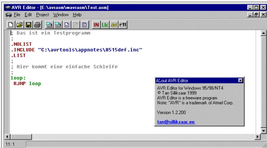
The editor recognizes instructions automatically and uses different colors (syntax highlighting) to signal user constants and typing errors in those instructions (in black). Storing the code in an .asm file provides nearly the same text file, colors are not stored in the file.
