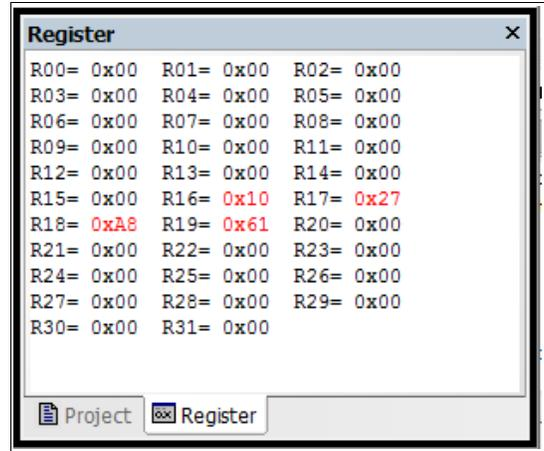
Multiplying the two MSBs (hex 27 and 61) and copying the result in R1:R0 to the two most upper result registers R5:R4 ...
