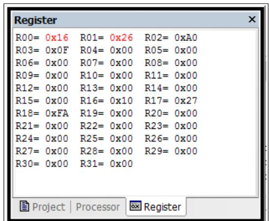
Now two steps are performed at once: multiplication by 256 and adding the result to the previous result. This is done by adding R1:R0 to Res3:Res2 instead of Res2:Res1. R1 can just be copied to Res3. R0 is added to Res2 then. If the carry is set after adding, the next higher byte Res3 is increased by one.
