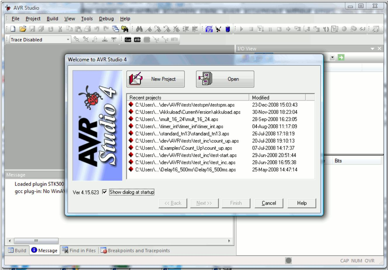
The first dialog asks whether an existing project should be opened or a new project is to be started. In case of a newly installed Studio “New Project” is the correct answer. The Button “Next>>” brings you to the settings dialog of your new project.
