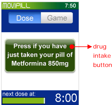
figure 6. MoviPill dose screen where patients inform medication intake. Drug intake data gathered by the phone was matched with ground truth data gathered by the MEMS pillbox to check if elders were pressing the button at the right time but taking the dose later on (game cheating).
