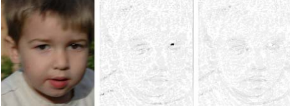
Figure 3. Original out of focus and motion blurred image, with specular highlight in the boy's left eye (left), amplified sharpness maps before contrast based correction (middle), and after contrast based correction (right).
