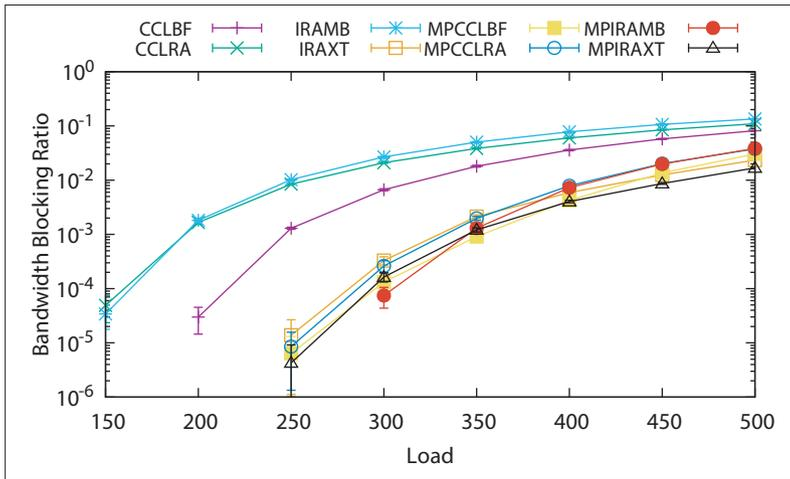
FIGURE 6. Bandwidth blocking ratio as function of the load for the USA topology.
