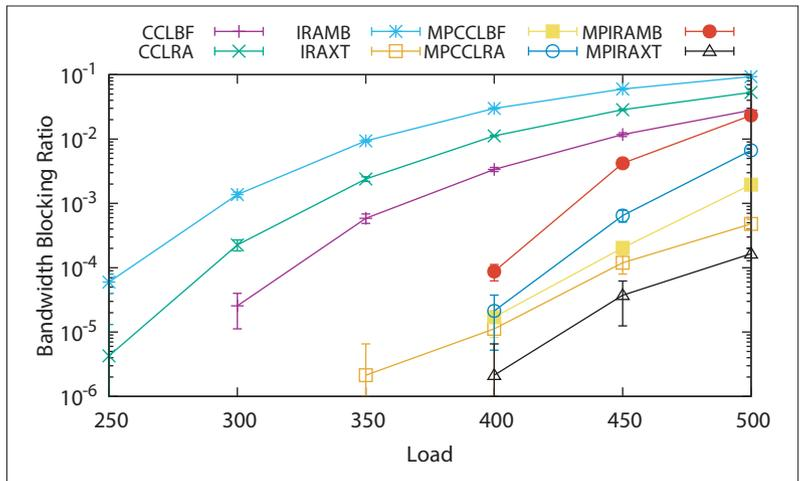
FIGURE 4. Bandwidth blocking ratio as function of the load for the NSF topology.
