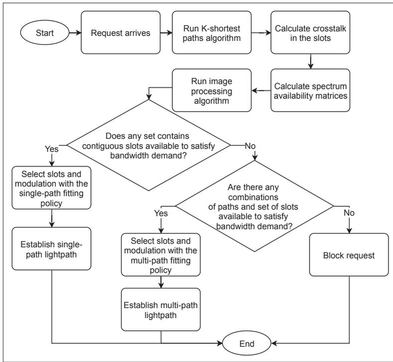
FIGURE 2. Description of the multipath RCMLSA algorithms.
