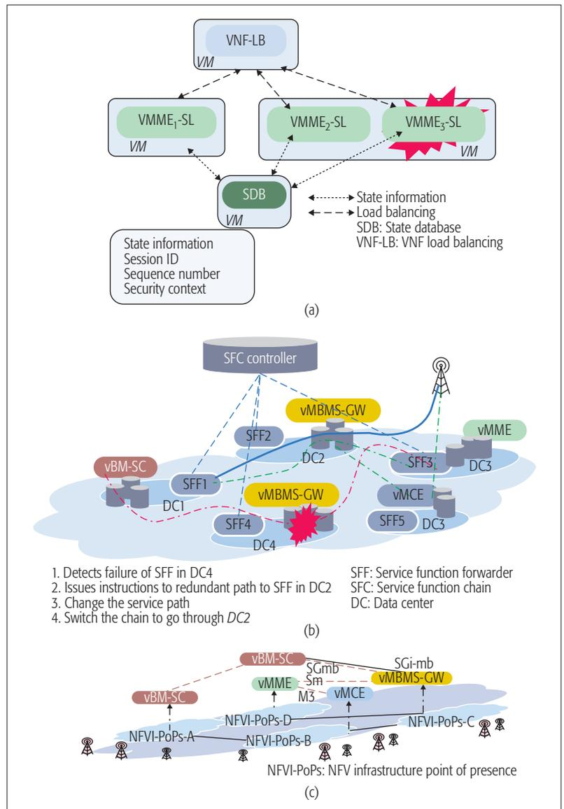
**Figure 3.** Example of the deployment of VNFs to provide resilience in an LTE-broadcasting service: a) service continuity with stateful VNF resilience; b) service resilience enabled by service function chain; c) service resilience provided by transparent topology with resources allocated in a multi-cloud environment in a geo-distributed location.
