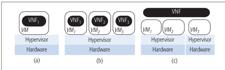
**Figure 2.** Deployment options for VNFs: a) VNF installed on a dedicated VM provided by the hypervisor; b) multiple VNFs hosted on the same physical host; c) multiple VNF components deployed in separate VMs on the same physical host or on a different physical host allocated in the cloud [12].
