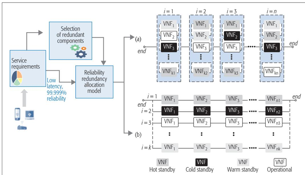
Figure 4. Reliability models with redundant VNF components for NFV deployment: a) Series-parallel; b) Parallel-series.
