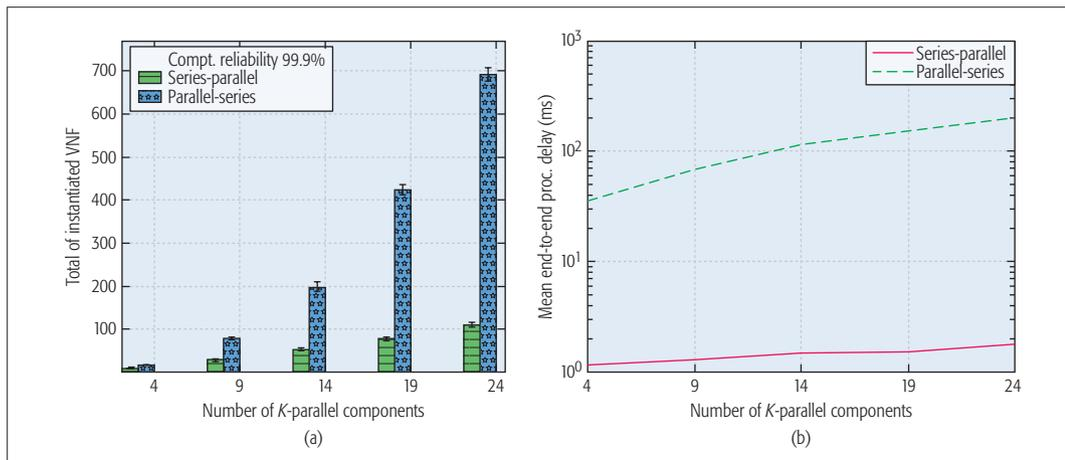
**Figure 5.** Comparison of the two redundancy models: a) the number of redundant VNFs instantiated in series-parallel and parallel-series models; b) the end-to-end delay service in series-parallel and parallel-series models.
