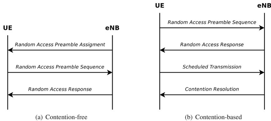
Figure 1. Random-access procedure in LTE-A networks
