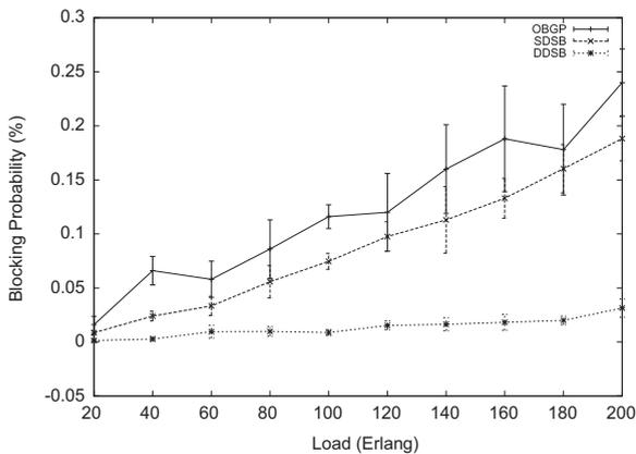
**Fig. 11.** Blocking probability as a function of the load for the NEWYORK topology.
