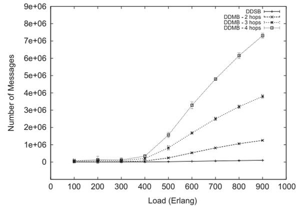
**Fig. 14.** Routing advertisements as a function of the load for DDSB and DDMB considering 2, 3 and 4 hops for the NOBEL-EU topology.
