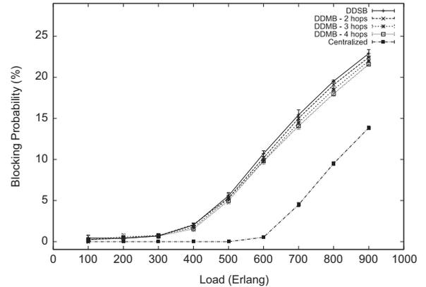
**Fig. 13.** Blocking probability as a function of the load for DDSB and DDMB considering 2, 3 and 4 hops for the NOBEL-EU topology.
