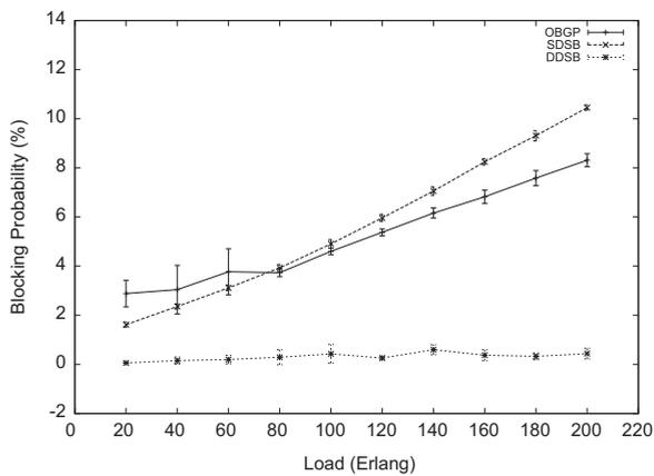
Fig. 8. Blocking probability as a function of the load for the NOBEL-EU topology.
