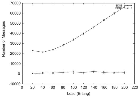
**Fig. 10.** Routing advertisements as a function of the load for the NOBEL-EU topology. Detailing the results for SDSB and DDSB.
