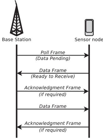
Fig. 4. SPP-MAC base station and sensor node transmission.
