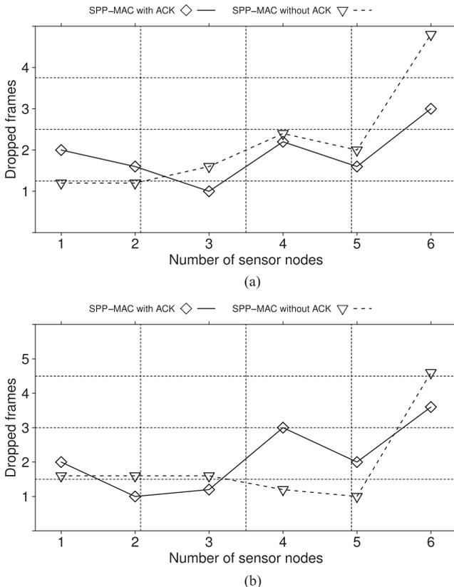
Fig. 15. Experimental dropped packets. (a) Traffic rate of 2 frames/s. (b) Traffic rate of 4 frames/s.
