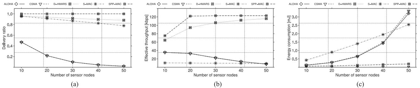
Fig. 8. Impact of the number of sensor nodes for the network using the same traffic rate. (a) Delivery ratio, (b) effective throughput, and (c) average energy consumption per bit.
