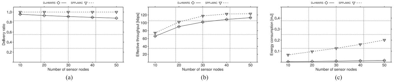
Fig. 11. Impact of the number of sensor nodes for the network using different traffic rate. (a) Delivery ratio, (b) effective throughput, and (c) average energy consumption per bit.
