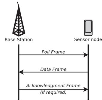
Fig. 2. SPP-MAC sensor node transmission.
