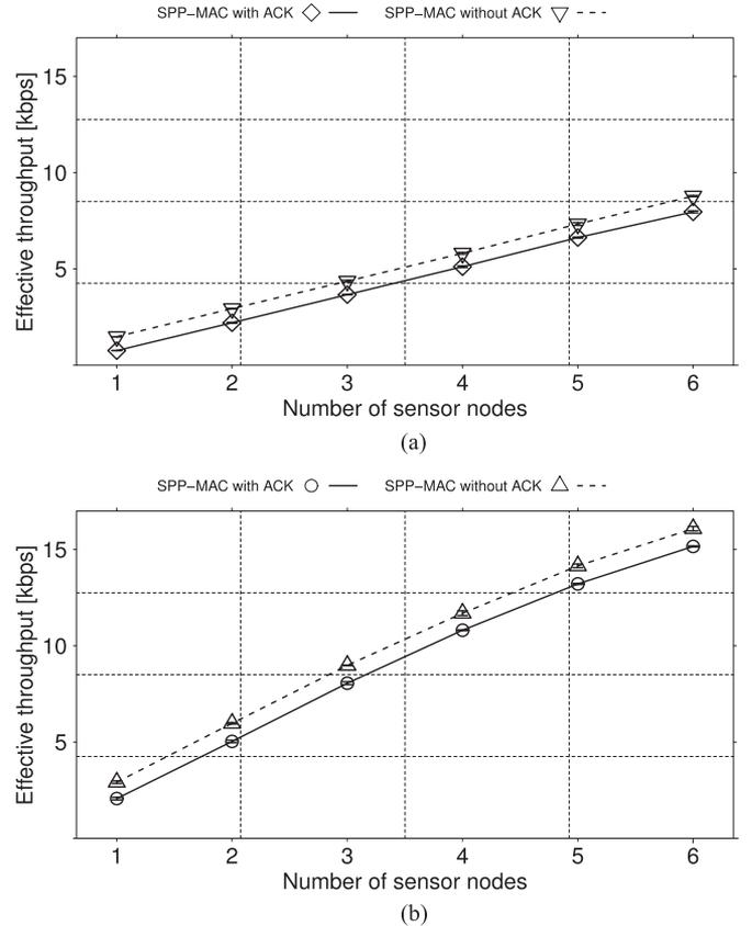
Fig. 13. Experimental effective throughput. (a) Traffic rate of 2 frames/s. (b) Traffic rate of 4 frames/s.
