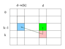
$$z[k,d] = max \{ z[k-1,d] , z[k-1,d-w[k]] + c[k]$$
