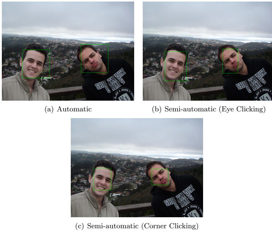
Figure 10: Different types of face location. Automatic and semi-automatic locations select a considerable background part, whereas manual location is restricted to face region.
