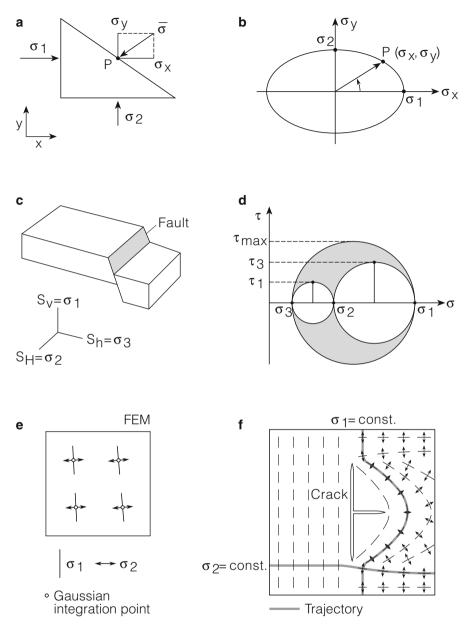
**Fig. 2.8** Visualizing stress in physical space (*left*) and stress space (*right*). The relationship in 2D between a Cartesian frame and principal stresses (**a**) is shown by a stress ellipse (**b**). The relationship in 3D between a Mohr frame (normal and shear stress) and principal stresses of a normal fault in the Earth's crust (**c**) is shown by a Mohr circle of stress (**d**). Principal stress directions at points (**e**) are shown as stress trajectories (**f**)
