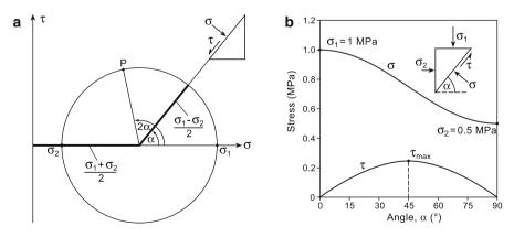
**Fig. 2.7** Mohr circle of stress **a** in *stress space*, and **b** in *physical space*. The Mohr circle relates principal stresses ( $\sigma_1$ ,  $\sigma_2$ ) to normal and shear stresses on an arbitrary tilted plane ( $\sigma$ ,  $\tau$ ,  $\alpha$ ) inside a deformable body
