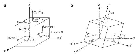
**Fig. 2.4** Visualization of stress components in 3D on a cube **a** before and **b** after solving the eigenvalue problem of the stress matrix; engineering mechanics notation (tension positive convention)
