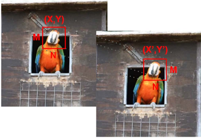
Fig. 2. Example of a macroblock and its respective Motion Vector between the current frame (left) and the reference frame (right). The original images are under Creative Commons Licence.
