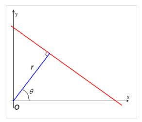
The parameter r represents the distance between the line and the origin, while  $\theta$  is the angle of the vector from the origin to this closest point (see Coordinates). Using this parameterization, the equation of the line can be written as [4]
