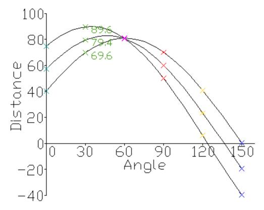
The point where the curves intersect gives a distance and angle. This distance and angle indicate the line which intersects the points being tested. In the graph shown the lines intersect at the pink point; this corresponds to the solid pink line in the diagrams above, which passes through all three points.
