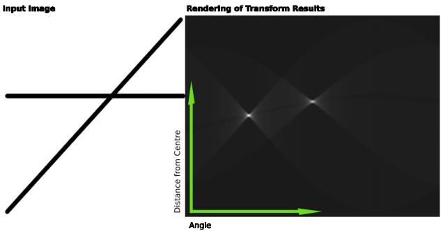
The results of this transform were stored in a matrix. Cell value represents the number of curves through any point. Higher cell values are rendered brighter. The two distinctly bright spots are the Hough parameters of the two lines. From these spots' positions, angle and distance from image center of the two lines in the input image can be determined.
