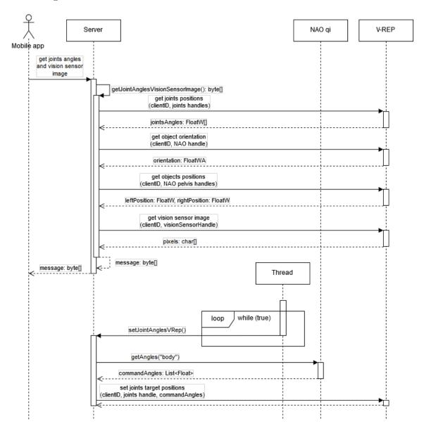
Figure 4: Get joints angles and vision sensor image sequence diagram
