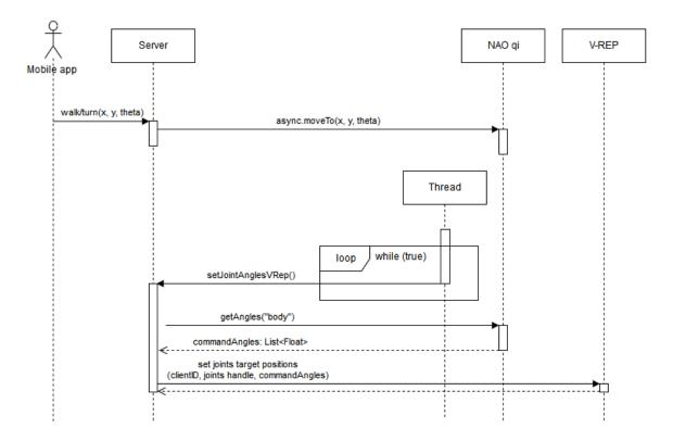
Figure 5: Walk/turn sequence diagram
