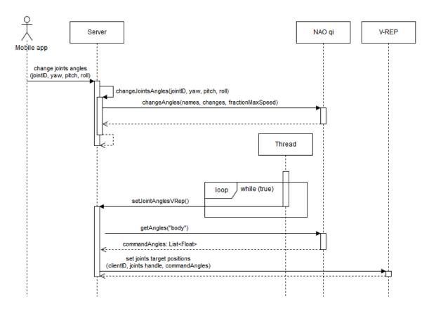
Figure 7: Change joints angles sequence diagram
