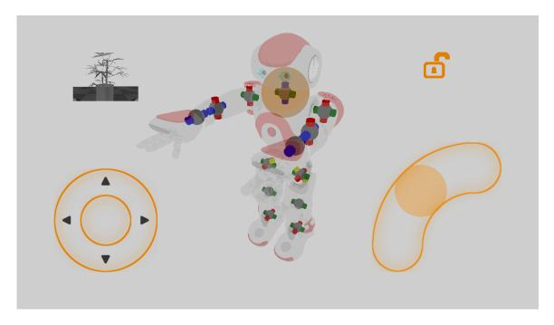
Figure 13: Individual joints adjustment operation mode with the head joint selected
