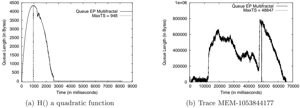
Figure 5: MaxTS for both synthetic and real network traffic
