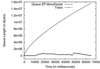
Figure 6: MaxTS estimated using monofractal EP for real network traffic
