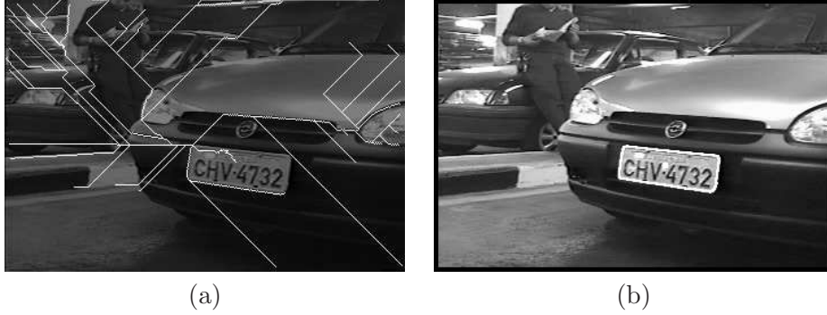
Figure 9: Example of license plate segmentation. (a) The original image overlaid by the number of descendants in the background set \mathcal{B} . (b) The resulting segmentation with tree pruning.
