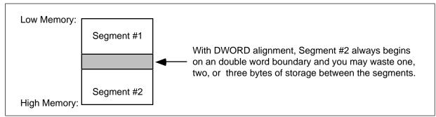
Figure 8.3 Segment with DWord Alignment
