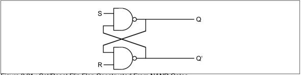
Figure 2.21 : Set/Reset Flip Flop Constructed From NAND Gates
