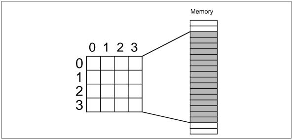
Figure 5.2 Mapping a 4 x 4 Array to Memory
