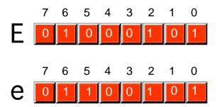
Figure 1.14: ASCII Codes for "E" and "e".
