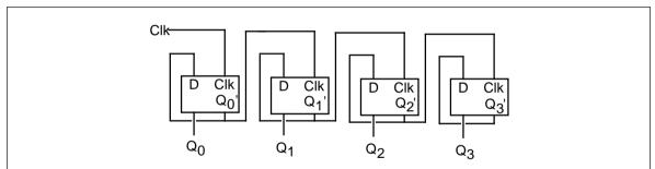
Figure 2.25 : A Four-bit Counter Built from D Flip-flops
