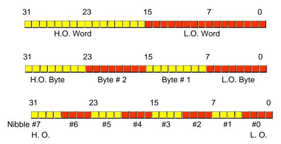
Figure 1.7: Nibbles, Bytes, and Words in a Double Word
