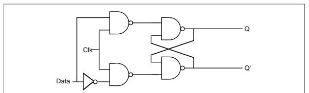
Figure 2.22 : Implementing a D flip-flop with NAND Gates
