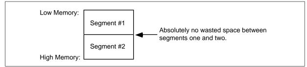
Figure 8.1 Segment with Byte Alignment
