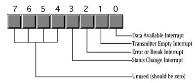
Serial Port Interrupt Enable Register (IER)
