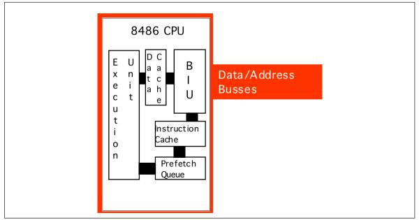
Figure 3.28 Internal Structure of the 8486 CPU
