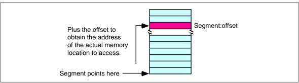
Figure 4.5 Segmented Addressing in Physical Memory
