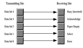
Connections on a Laplink Compatible Cable
