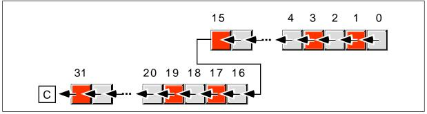
Figure 8.3 32-bit Shift Left Operation
