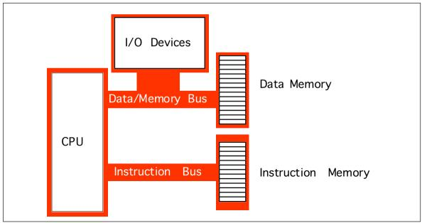
Figure 3.27 A Typical Harvard Machine
