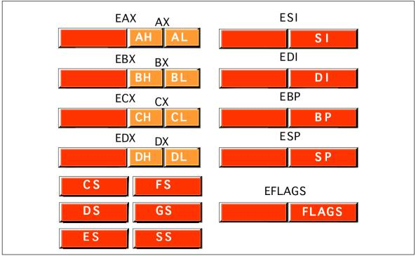
Figure 4.3 80386 Registers (Application Programmer Visible)
