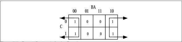
Figure 2.6 : Correct Rectangle for the Function
