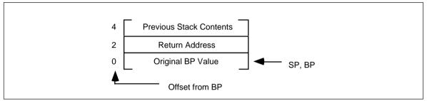
Figure 11.13 Stack Upon Entry into the ForStmt Procedure
