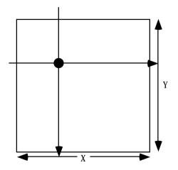
A joystick uses two independent pots to provide an (X,Y) input value. Horizontal movements on the joystick affect the x-axis pot independently of the y-axis pot. Likewise, vertical movements affect the y-axis pot independent of the x-axis pot. By reading both pots you can determine the position of the joystick in the (X,Y) coordinate system.
