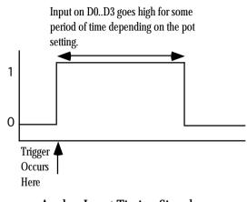
The only remaining question is "how do we determine the length of the pulse?" The following short loop demonstrates one way to determine the width of this timing pulse:
