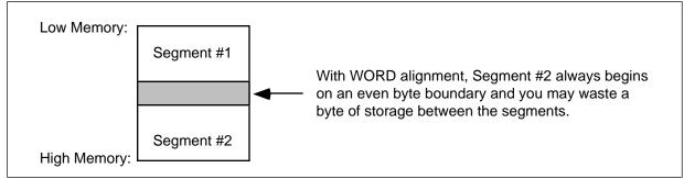
Figure 8.2 Segment with Word Alignment
