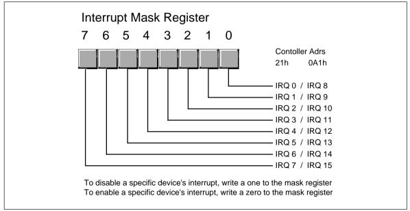
Figure 17.1 8259 Interrupt Mask Register
