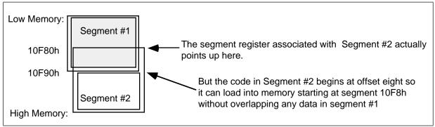
Figure 8.6 Paragraph Alignment of Segments
