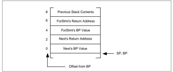
Figure 11.15 The Stack upon Entering the Next Procedure
