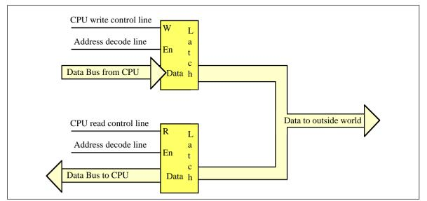
Figure 3.33 An Input/Output Port Requires Two Latches
