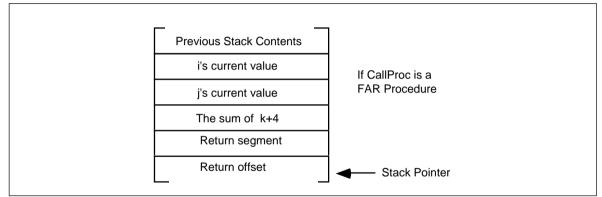
Figure 11.6 CallProc Stack Layout for a Far Procedure
