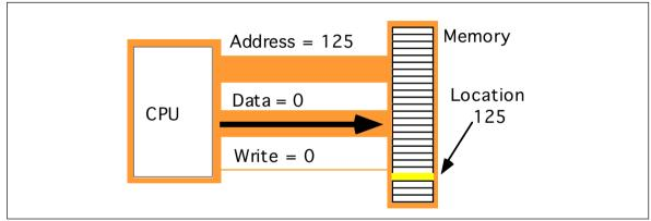
Figure 3.2 Memory Write Operation
