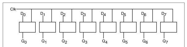
Figure 2.23 : An Eight-bit Register Implemented with Eight D Flip-flops
