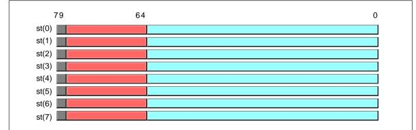
Figure 14.5 80x87 Floating Point Register Stack
