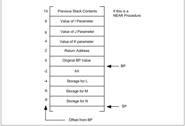
Figure 11.16 The Stack upon Entering the Next Procedure
