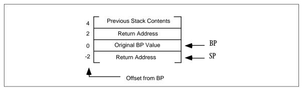
Figure 11.14 Stack Just Before Leaving the ForStmt Procedure
