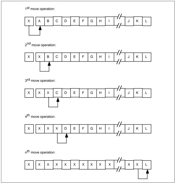
Figure 15.1 Overwriting Data During a Block Move Operation
