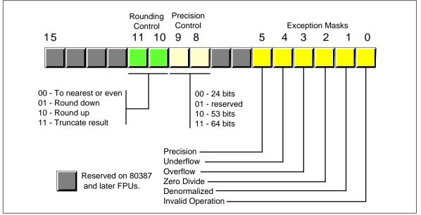
Figure 14.6 80x87 Control Register
