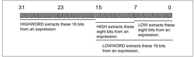
Figure 8.7 HIGHWORD, LOWWORD, HIGH, and LOW Operators
