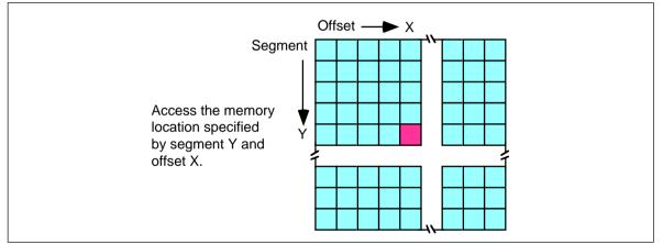
Figure 4.4 Segmented Addressing as a Two-Dimensional Process
