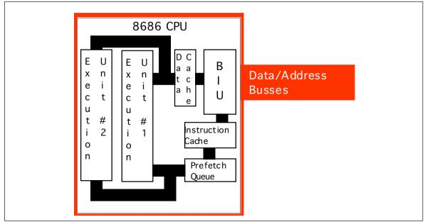
Figure 3.31 Internal Structure of the 8686 CPU
