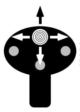
The cooley switch (shown here on a device layout similar to the CH Products' FlightStick Pro) is a thumb actuated digitial joystick. You can move the switch up, down, left or right, activating individual switches inside the game input device.
