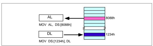
Figure 4.8 Displacement Only (Direct) Addressing Mode
