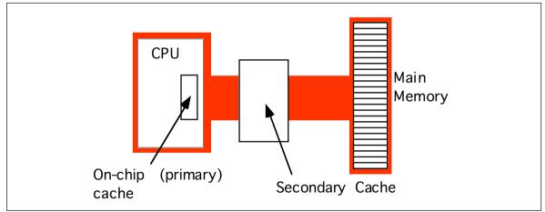
Figure 3.15 A Two Level Caching System
