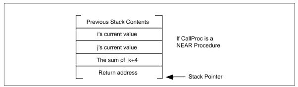
Figure 11.5 CallProc Stack Layout for a Near Procedure
