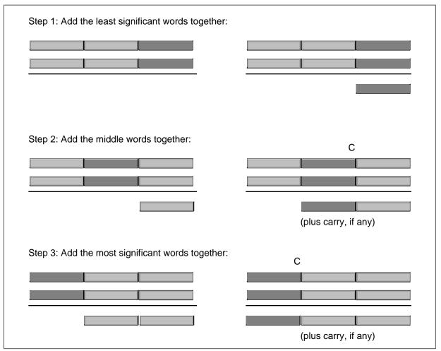
Figure 8.1 Multiprecision (48-bit) Addition
