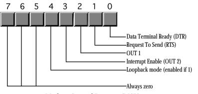
Modem Control Register (MCR)
