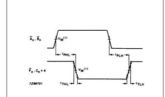
Fig.9 Propagation delays for operands to carry output and function outputs.
