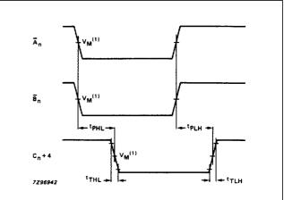
Fig.10 Propagation delays for operands to carry output.
