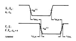
Fig.7 Propagation delays for carry input to carry output, carry input to function outputs, operands to carry generate operands, propagation outputs and output transition lines.
