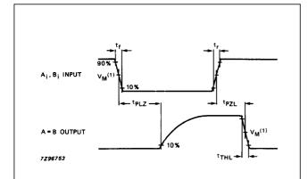
Fig.11 Waveforms showing the input (A<sub>i</sub>, B<sub>j</sub>) to output (A=B) propagation delays and output transition time of the open drain output (A=B).
