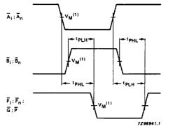
Fig.8 Propagation delays for operands to carry generate, propagate outputs and function outputs.
