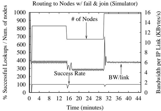
Fig. 19. *Route to Node under failure and joins.* The performance of Tapestry route to node with two massive network membership change events. Starting with 830 nodes, 20% of nodes (166) fail, followed 16 minutes later by a massive join of 50% (333 nodes).
