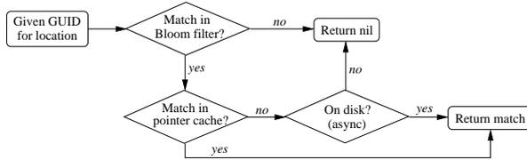
Fig. 9. *Enhanced Pointer Lookup*. We quickly check for object pointers using a Bloom filter to eliminate definite non-matches, then use an in-memory cache to check for recently used pointers. Only when both of these fail do we (asynchronously) fall back to a slower repository.
