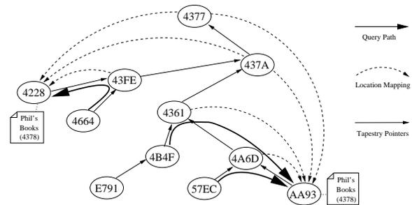
Fig. 5. *Tapestry route to object example.* Several nodes send messages to object 4378 from different points in the network. The messages route towards the root node of 4378. When they intersect the publish path, they follow the location pointer to the nearest copy of the object.
