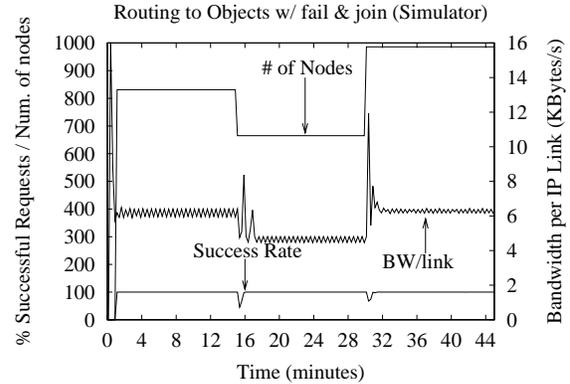
Fig. 20. *Route to Object under failure and joins.* The performance of Tapestry route to objects with two massive network membership change events. Starting with 830 nodes, 20% of nodes (166) fail, followed 16 minutes later by a massive join of 50% (333 nodes).
