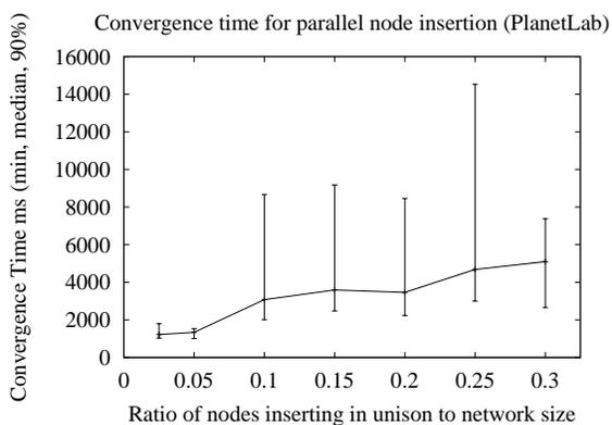
Fig. 18. *Parallel Insertion Convergence*. Time for the network to stabilize after nodes are inserted in parallel, as a function of the ratio of nodes in the parallel insertion to size of the stable network.
