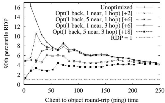
Fig. 15. 90<sup>th</sup> percentile RDP of Routing to Objects with Optimization. Each line represents a set of optimization parameters ( $k$  backups,  $l$  nearest neighbors,  $m$  hops), with cost (additional pointers per object) in brackets.
