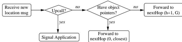
Fig. 7. *Message processing.* Object location requests enter from neighbor link layer at the left. Some messages are forwarded to an extensibility layer; for others, the router first looks for object pointers, then forwards the message to the next hop.
