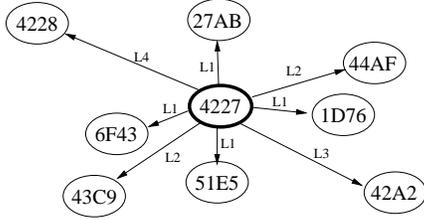
Fig. 1. *Tapestry routing mesh from the perspective of a single node.* Outgoing neighbor links point to nodes with a common matching prefix  $x$ . Higher-level entries match more digits. Together, these links form the local routing table.
