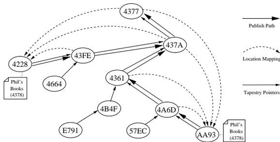
Fig. 4. *Tapestry object publish example.* Two copies of an object (4378) are published to their root node at 4377. Publish messages route to root, depositing a location pointer for the object at each hop encountered along the way.
