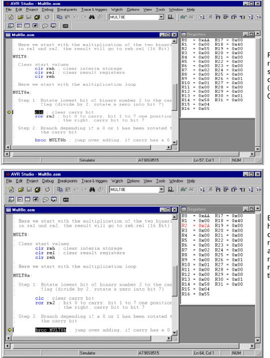
R2 is rotated to the right, to roll the least significant bit into the carry bit. 0x55 (0101.0101) yielded 0x2A (0010.1010).
