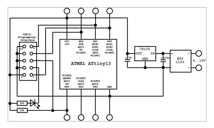
The ATtiny13 requires no external XTAL or clock generator, because it works with its internal 9.6 Mcs/s
