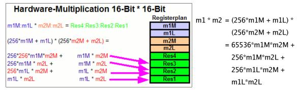
Obviously four multiplications now. We start with the first and the last as the two easiest ones: their results are simply copied to the correct result register positions. The results of the two multiplications in the middle of the formula have to be added to the middle of our result registers, with possible carry overflows to the most significant byte of the result. To do that, you will see a simple trick that is easy to understand. The software:
