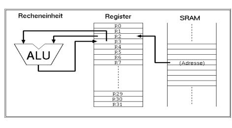
Unit ALU, sometimes called accumulator) like the registers are. If you access these memory locations you usually use a register as interim storage. In the example displayed here a value in SRAM will be copied to the register R2 (1st instruction), a calculation with the value in R3 is made and the result is written R3 (second to instruction). After that this value is written back to the same SRAM location (instruction 3, not shown here).
