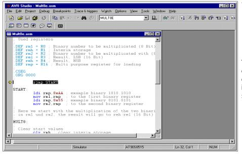
The object-code has been opened, the cursor is placed on the first executable instruction. F11 does single steps.
