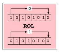
For understanding the multiplication operation, it is necessary to understand the binary rotation instructions ROL and ROR. These instructions shift all bits of a register one position left (ROL) resp. right (ROR). The void position in the register is filled with the content of the carry bit in the status register, the bit that rolls out of the register is shifted to this carry bit. This operation is demonstrated using 0xAA as an example for ROL and 0x55 as an example for ROR.
