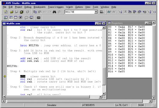
Now the register pair R1:R0 is rotated one position left to multiply this binary by 2. From 0x00AA, multiplication by 2 yields 0x0154.
