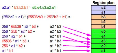
The multiplication of a 16 bit binary "a" with a 24 bit binary "b" leads to results with up to 40 bit length. The multiplication scheme requires six 8-by-8-bit multiplications and adding the results to the appropriate position in the result registers.
