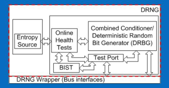
A reusable IP module that provides each embedding with an autonomous/self contained, high quality/high performance, "complete" DRNG
