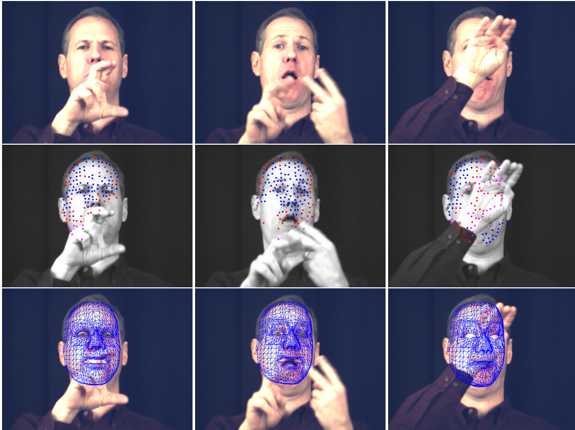
Figure 4. Snapshots of a tracking sequence. Top to bottom: original sequence, categorized image correspondences, final 3D model position. The correspondences constitute a mix of KLT and edge tracking results. In the center row, blue points denote accepted correspondences, red points denote rejected outliers, and purple points denote correspondences eliminated by optical flow thresholding.
