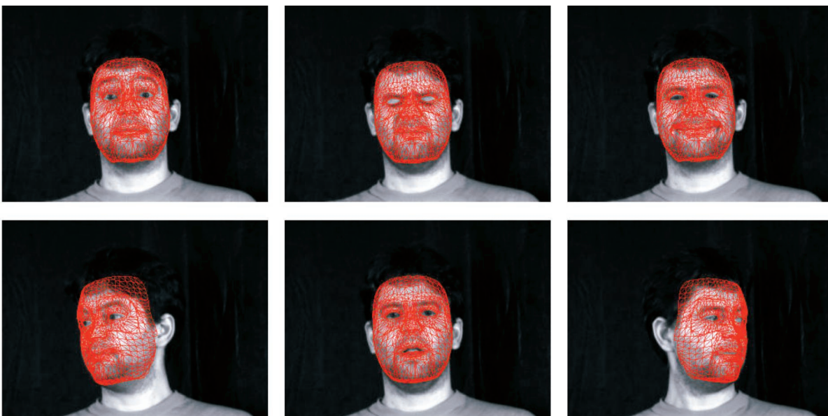
Fig. 4. Six snapshots of a tracking sequence of 3,600 frames. The deformable model used here has 11 parameters.
