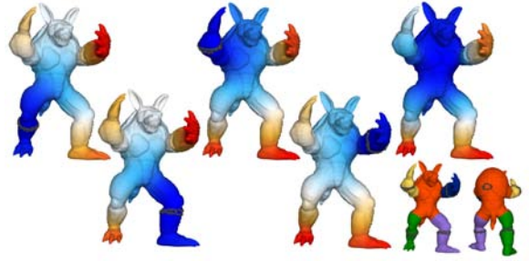
Figure 3: Front propagation from each medial structure. Spheres indicate the points of the medial structures. Colors encode the iso-values of the diffusion distance between the medial structures and the surface points, ranging from blue to red. Note that the colors change greatly in the concavities.
