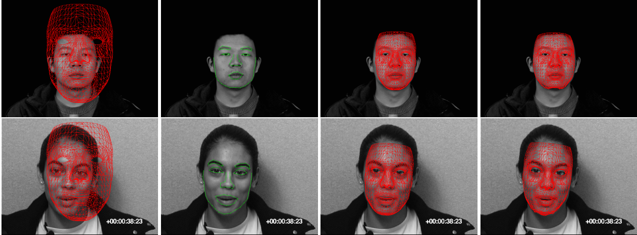
Figure 5. Automated model fitting and adaptation. Left to right: Before model fitting, ASM feature detection, Adjustment of rigid model parameters, Final fit after adjustment of nonrigid shape parameters.
