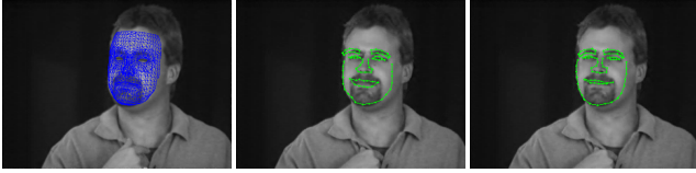
Figure 4. 3D model-guided ASM initialization. Left to right: Tracked model position from previous frame. Initial ASM guess in next frame, based on model position from previous frame. Final ASM shape in next frame.
