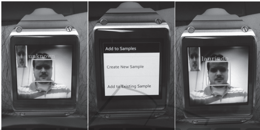
Figure 2: Gear Face Recognition: an unknown person (left), adding a sample (center) and a recognized person (right).
