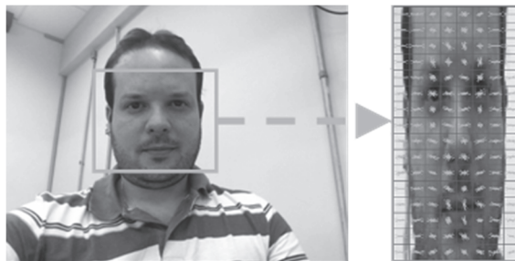
Figure 1: Example of image conversion in HOG descriptor.
