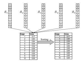
Figure 5: Example of the application of the voting scheme.
