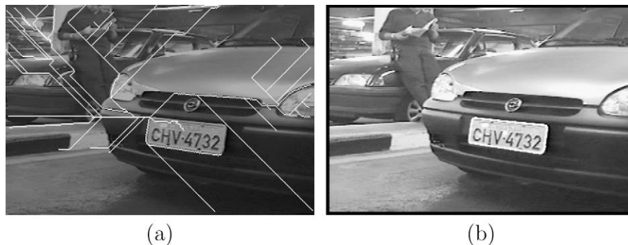
Fig. 9. Example of license plate segmentation. (a) The original image overlaid by the number of descendants in the background set \mathcal{B} . (b) The resulting segmentation with tree pruning.
